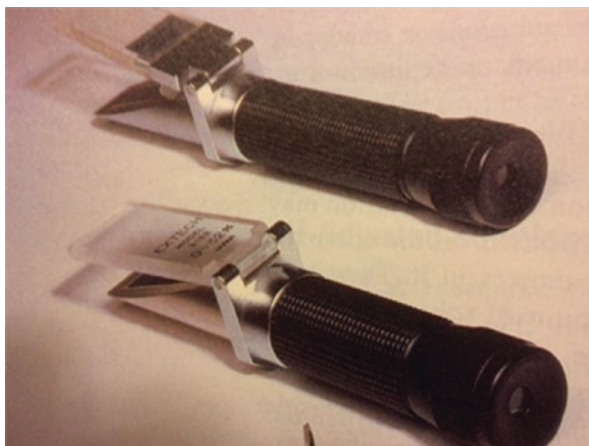
Fig. 10.1 Two similar types of refractometer, or total solids meter
