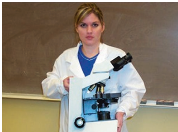
Fig. 17.3 Proper transport of the microscope to avoid damage by dropping
