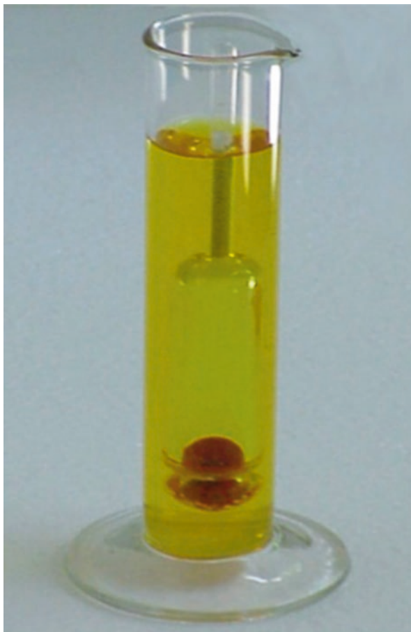
Fig. 10.3 Urinometer, a special glass cylinder with flotation device
